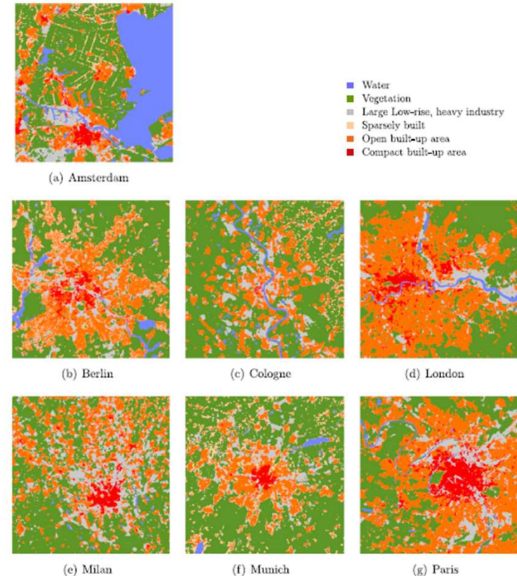
Fig. 12. Land cover maps produced for the seven cities. To present an equivalent size for all test cases, only a part of each city map, covering about 39.7 \times 39.7 km 2 , is shown. The GSD of each map is 50 m.
